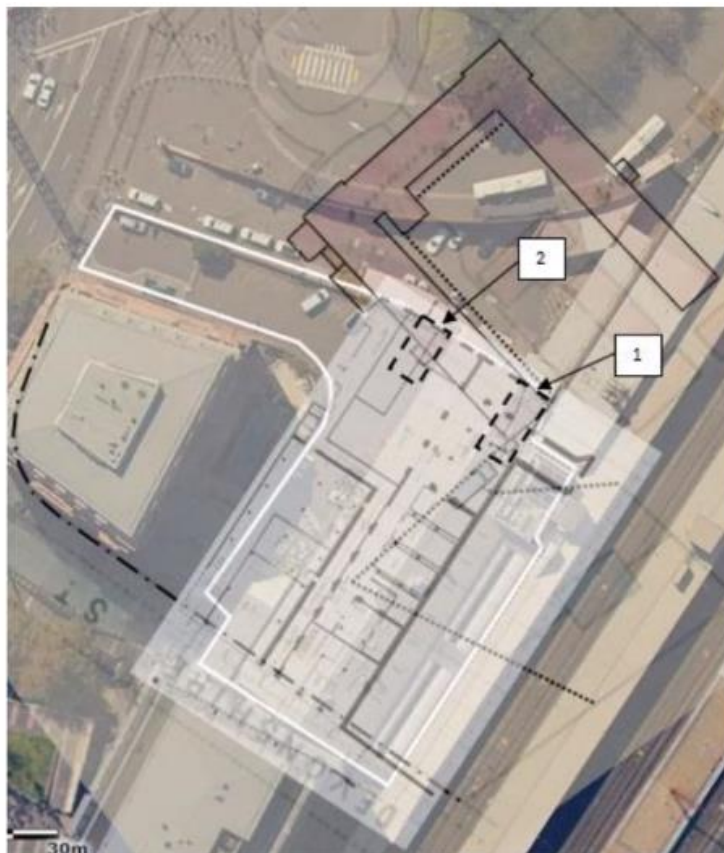
Figure 7.1 Proposed test trench locations overlaid with extant building plan. Where internal walls and columns are located within the trench the excavation will avoid these structures.
