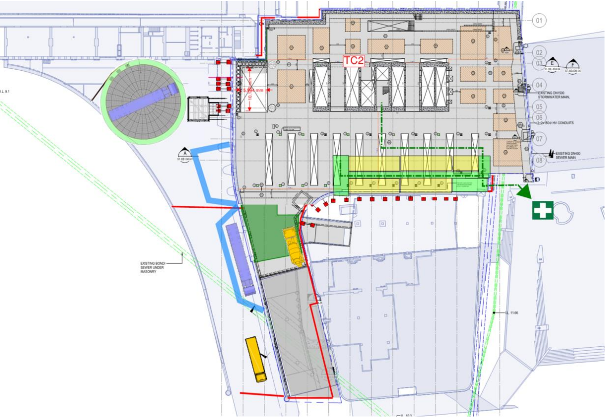
Figure 1.39c: Phase 3 – tower construction egress pathway
