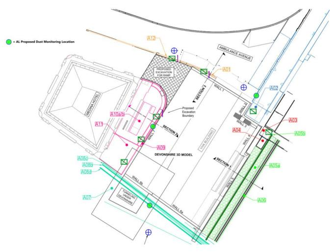
**Figure 7: Recommended Dust Monitoring Locations**
