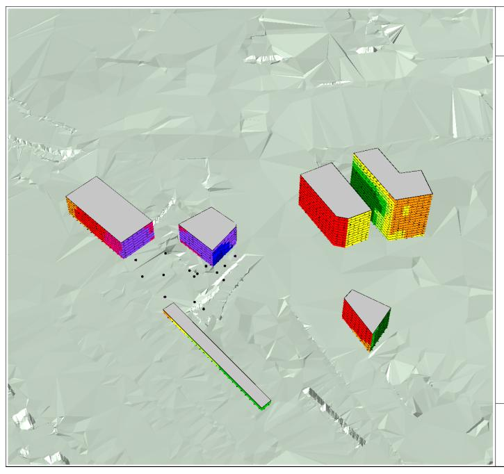
Predicted Excavation and Piling Noise Levels
