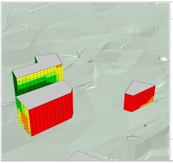
Predicted Excavation and Piling Noise Levels
