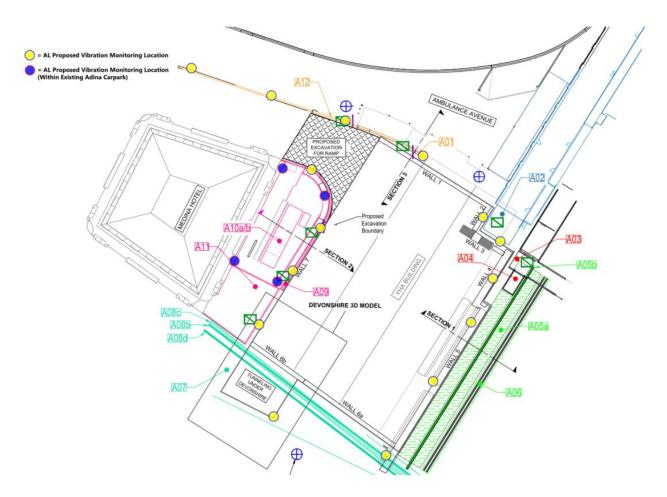
**Figure 6: Recommended Vibration Monitoring Locations**
