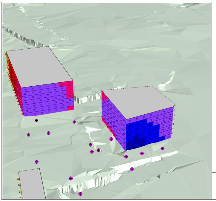
Predicted Excavation and Piling Noise Levels
