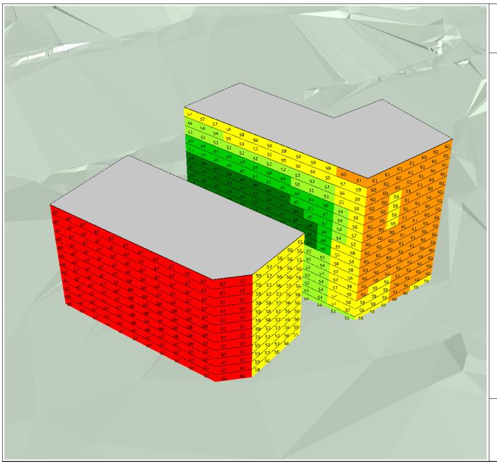
Predicted Excavation and Piling Noise Levels
