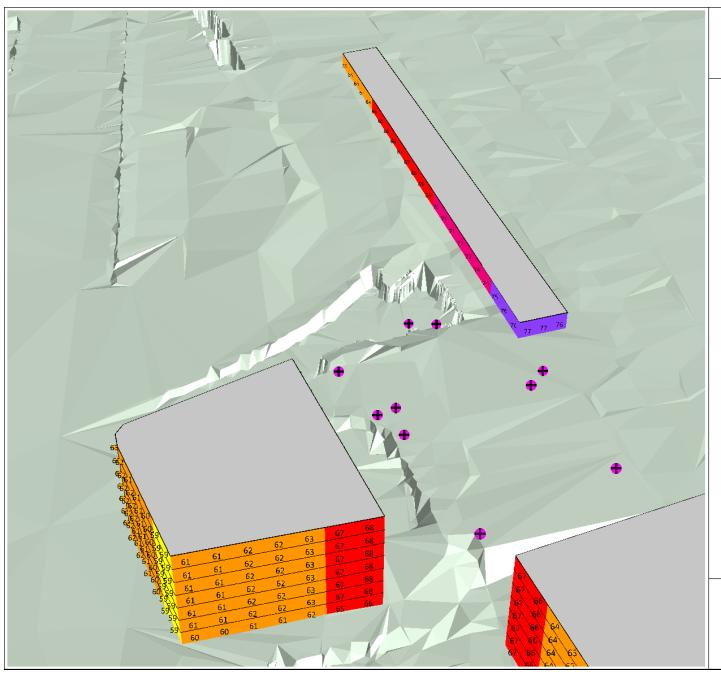
Predicted Excavation and Piling Noise Levels
