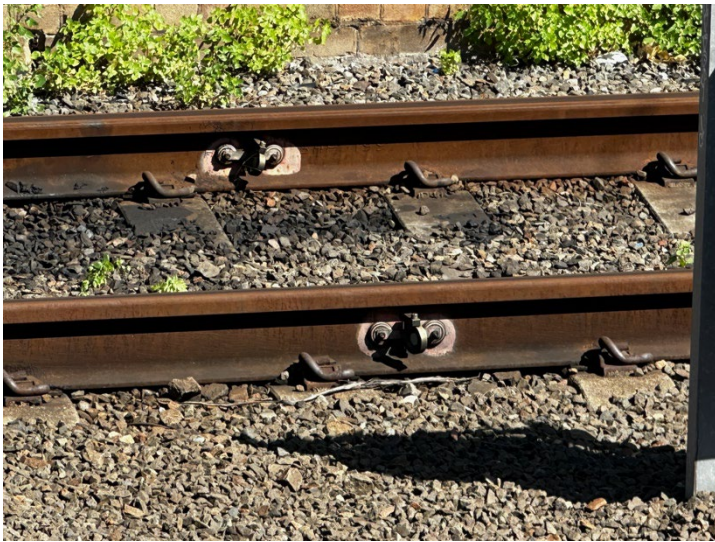
Photo 11: Movement monitors placed on adjacent rail track
